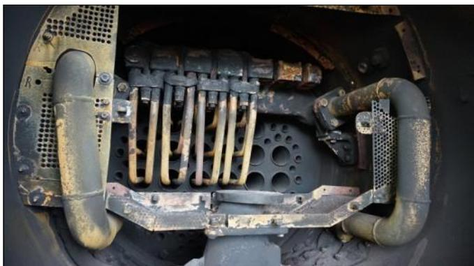
Just to recap on what these units actually do, hidden away there in the boiler. Basic steam engines use what is known as 'saturated steam', that is steam created directly from heat, as in a kettle but under pressure.
